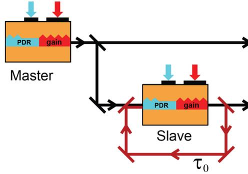
Fig. 1 – (Color online) Setup of master and slave DFB lasers with PDR for realization of anticipated synchronization.
