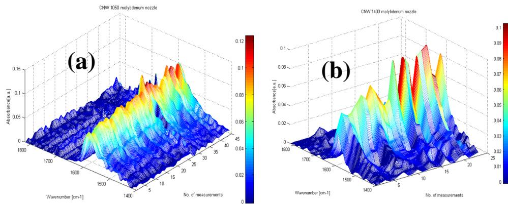
Fig. [6] - Ageing FTIR spectra of carbon nanowalls samples: 1400-1800  $\text{cm}^{-1}$  range for (b) CNW 1050 sccm; (c) CNW 1400 sccm.
