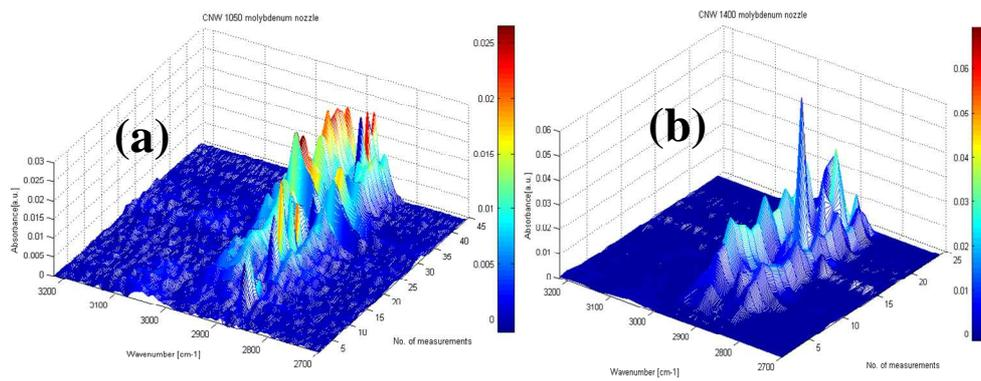
Fig. [7] - Ageing FTIR spectra of carbon nanowalls samples: 2700-3200  $\text{cm}^{-1}$  range for (b) CNW 1050 sccm; (c) CNW 1400 sccm.
