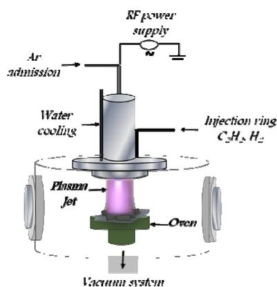
Fig. [1] - The experimental setup showing the deposition chamber.
