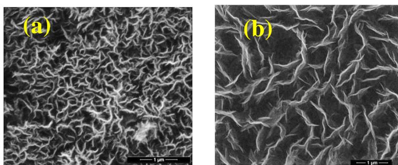
Fig. [2] - SEM images: (a) CNW 1050 sccm; (b) CNW 1400 sccm.
