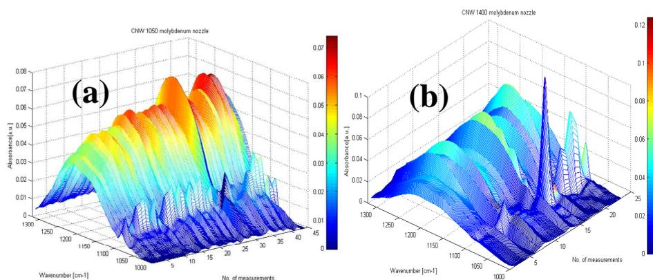
Fig. [5] - Ageing FTIR spectra of carbon nanowalls samples: 1000-1300  $\text{cm}^{-1}$  range for (b) CNW 1050 sccm; (c) CNW 1400 sccm.
