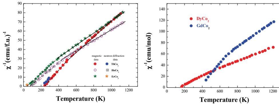
Fig. 5 – Thermal variations of reciprocal susceptibilities for  $R\text{Co}_2$  compounds with: a)  $R = \text{Tb}, \text{Ho}, \text{Er}$ ; b)  $R = \text{Gd}, \text{Dy}$ . The magnetic susceptibilities determined from polarized neutron studies, in the temperature range  $T_c < T < 300$  K are as also given.
