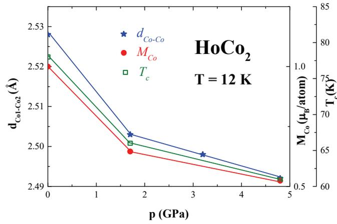
Fig. 1 – Pressure dependences of the distances between cobalt atoms, cobalt moments and Curie temperatures, in  $HoCo_2$  compound.
