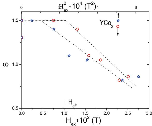
Fig. 8 – The cobalt spin values determined from saturated effective moments in  $\text{RCO}_2$  compounds on exchange field,  $H_{\text{ex}}$  ( $\circ$ ) or square of exchange field  $H_{\text{ex}}^2$  ( $\star$ ) acting on cobalt in  $\text{RCO}_2$  compounds, at  $T = 4$  K.
