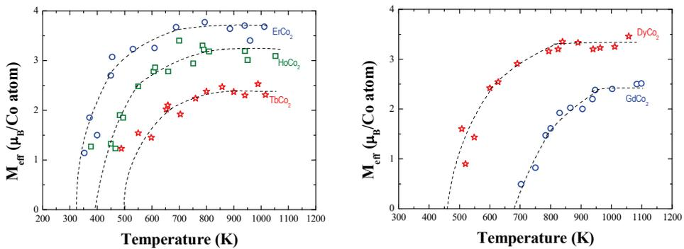
Fig. 6 – Thermal variations of the effective cobalt moments, at  $T > T_1$ , for  $\text{RCo}_2$  compounds with:
