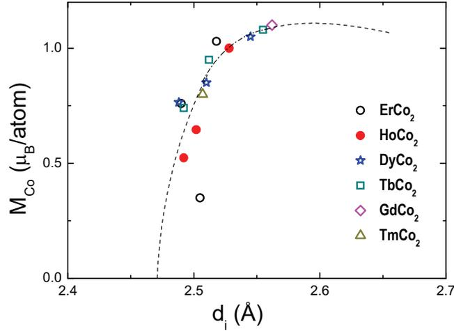
Fig. 2 – The dependence of cobalt moments on the distances  $d_i$  between the cobalt atoms as determined from pressure studies. By broken lines is denoted the Néel-Slater curve.
