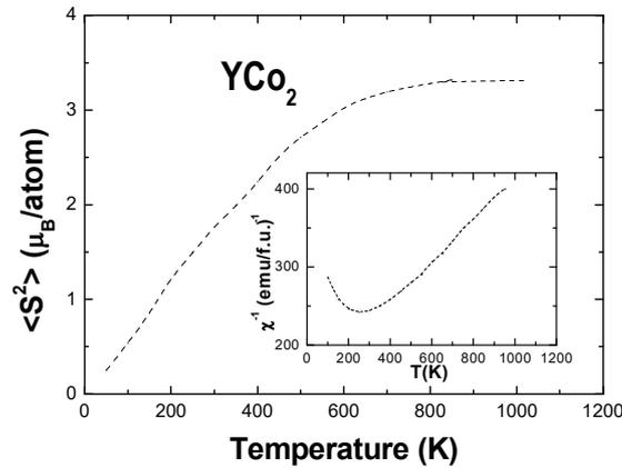
Fig. 7 – Temperature dependence of the mean square amplitude of spin fluctuations in  $\text{YCo}_2$ . In inset is shown the thermal variation of reciprocal susceptibility.
