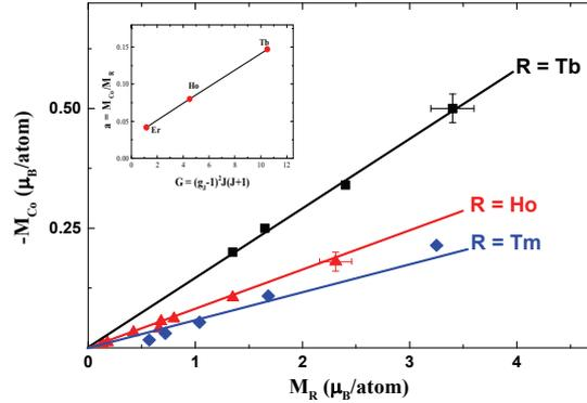
Fig. 4 – The dependences of cobalt moments on the rare-earth ones in  $R\text{Co}_2$  compounds with  $R = \text{Tb}, \text{Ho}, \text{Tm}$  at  $T > T_c$ . For each compound, linear trend is evidenced, not dependent on the external field and temperature. In inset is shown the rates of the above dependences as function of De Gennes factor.
