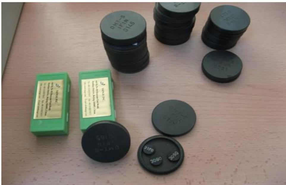
Fig. 1 – Dosimetry box with thermoluminescent detectors.
