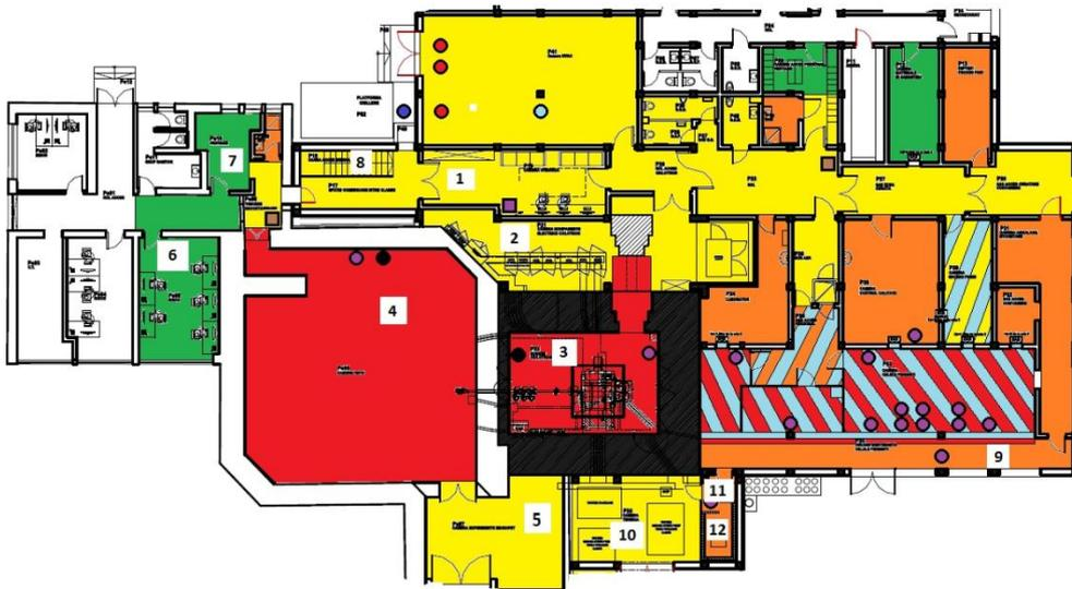
Fig. 2 – Schematic layout of the Radiopharmaceuticals Research Centre and the positions of the monitoring points.
