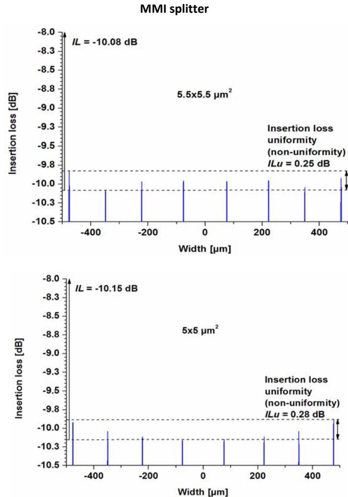
Fig. 3 – Detailed view of splitting parameters of  $1 \times 8$  Y-branch (left) and  $1 \times 8$  MMI (right) splitters with the waveguide core sizes of  $5.5 \times 5.5 \mu\text{m}^2$  (top) and  $5 \times 5 \mu\text{m}^2$  (bottom).
