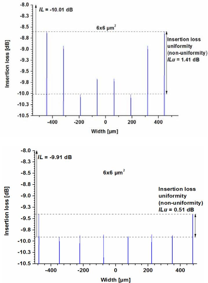
Fig. 2 – Top view of the simulated  $1 \times 8$  Y-branch (top-left) and MMI (top-right) structures. Field distribution at the end of  $1 \times 8$  Y-branch (middle-left) and  $1 \times 8$  MMI (middle-right) splitters. Non-uniformity and insertion loss of  $1 \times 8$  Y-branch (bottom-left) and  $1 \times 8$  MMI (bottom-right) splitters.
