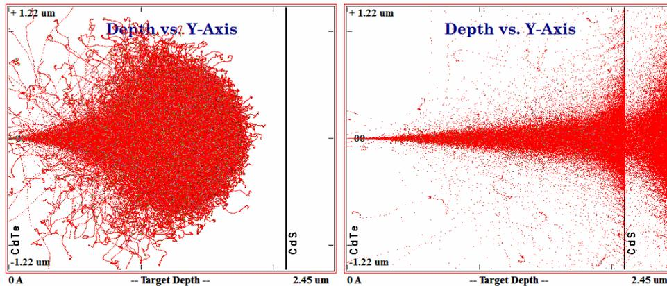
Fig. 2 – Spatial scattering distributions for alpha particles (left side) and protons (right side) with  $E = 500$  keV and  $F = 10^{11}$  particles/cm<sup>2</sup>. The numerical simulations were made taking into account a CdS/CdTe heterojunction; thickness of the component layers were 320 nm for CdS and 2.1  $\mu$ m for CdTe, respectively.
