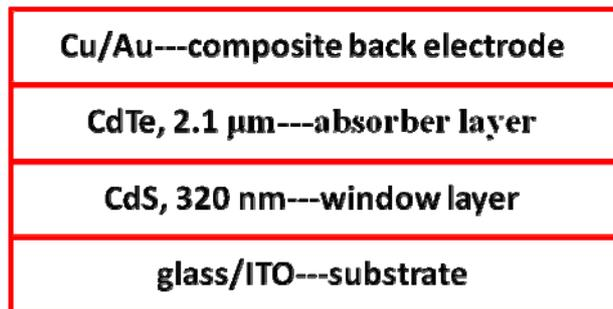
Fig. 1 – Fabricated cells architecture.
