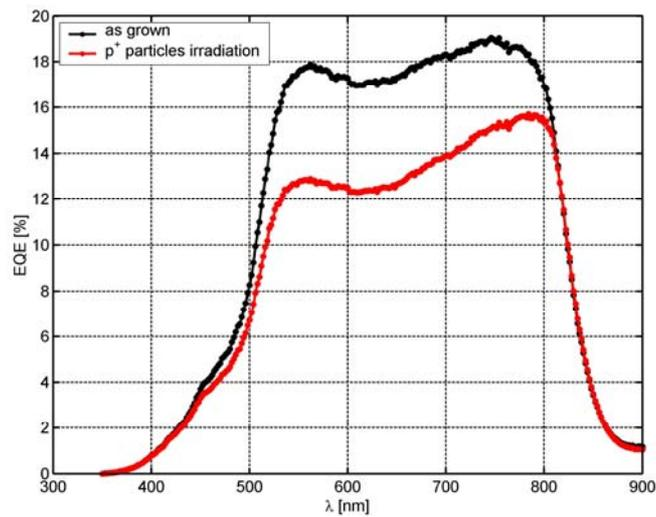
Fig. 3 – Action spectrum of external quantum efficiency of glass/ITO/CdS/CdTe/Cu/Au photovoltaic cells, as grown (black) and after irradiation with protons,  $E = 500$  keV,  $F = 10^{11}$  particles/cm<sup>2</sup> (red).
