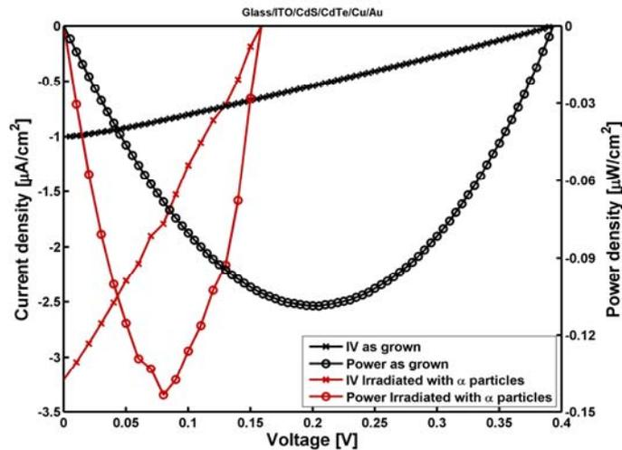
Fig. 6 – Current-voltage characteristics and power density of as grown glass/ITO/CdS/CdTe/Cu/Au photovoltaic cells (black) and after irradiation with alpha particles,  $E = 500$  keV,  $F = 10^{11}$  particles/cm<sup>2</sup> (red).
