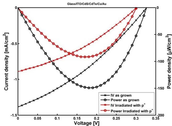
Fig. 4 – Current-voltage characteristics and power density of as grown glass/ITO/CdS/CdTe/Cu/Au photovoltaic cells (black) and after irradiation with protons,  $E = 500$  keV,  $F = 10^{11}$  particles/cm<sup>2</sup> (red).
