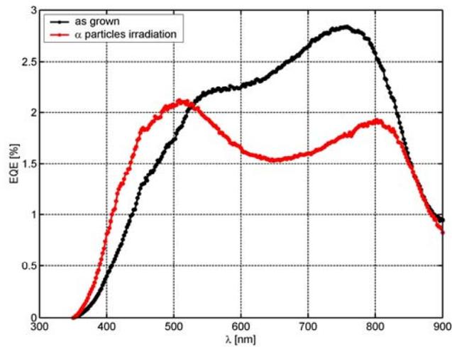
Fig. 5 – Typical EQE action spectra of glass/ITO/CdS/CdTe/Cu/Au photovoltaic cells before (black) and after irradiation with alpha particles,  $E = 500$  keV,  $F = 10^{11}$  particles/cm<sup>2</sup> (red).
