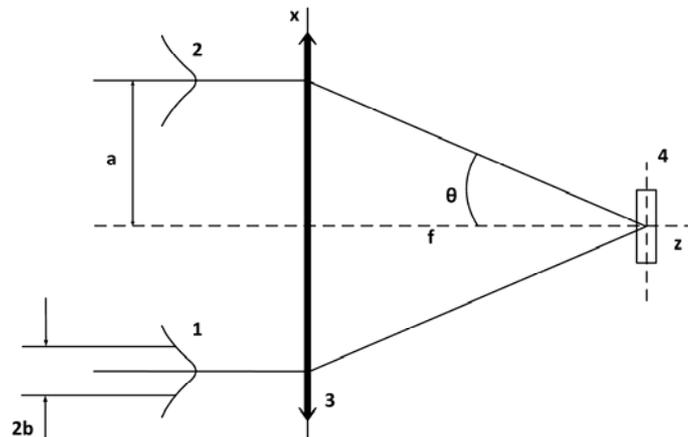
Fig. 2 – Schematic of the experimental setup: 1, 2 – input beams ( $b = 0.7$  mm) of semiconductor lasers ( $\lambda = 0.67$   $\mu\text{m}$ ), 3 – objective lens ( $f = 10$  mm), 4 – cell with tested particles suspended in water,  $a = 1.3$  mm,  $\theta = 7.4^\circ$ , NA = 0.16.
