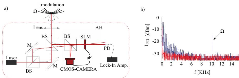
Fig. 2 – a) Setup of an CMOS-LCOS adaptive interferometer. The interference pattern is acquired by a CMOS camera and interferogram after signal processing, is sent to a LCOS-SLM. The light intensity diffracted by the the SLM is recorded by a photodiode; b) spectrum of the signal detected with a CMOS-LCOS at 10 KHz.
