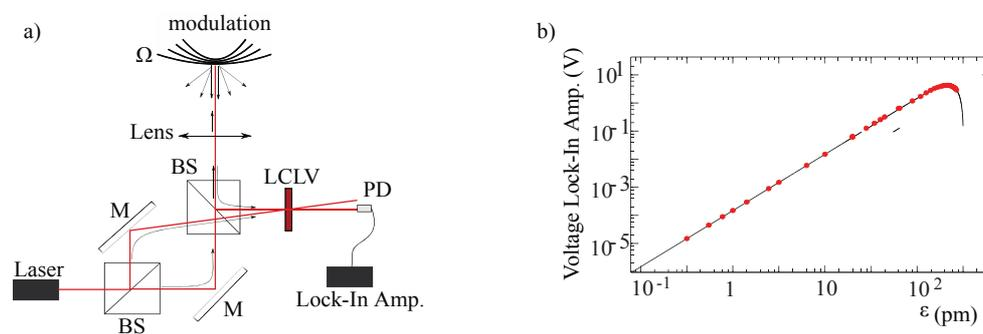
Fig. 1 – a) Adaptive holographic interferometer with LCLV. Reference and a signal beam interfere in the LCLV. The signal is a speckled beam resulting from the scattering from a vibrating object. The amplitude of the modulation is detected *via* a photodiode, PD; b) measured vibration amplitudes.
