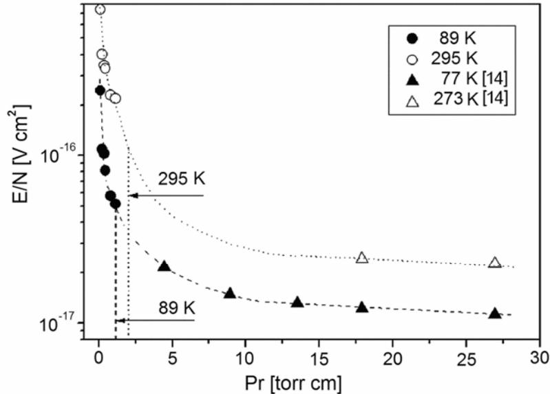
Fig. 2 – The reduced electric field  $E/N$  in a positive column *versus* the reduced pressure  $P_r$ , at cryogenic and room temperature at a discharge current  $I = 0.5$  mA. The arrow shows the border of dust plasma existence.
