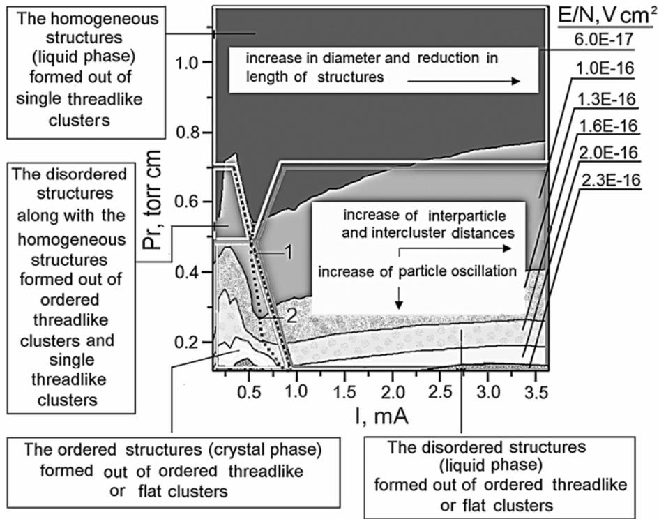
Fig. 5 – The diagram of state of dusty plasma in neon at  $T = 89$  K with isolines of the reduced longitudinal electric field strength: border of melting (1), border of the transition to the normal glow discharge (2).
