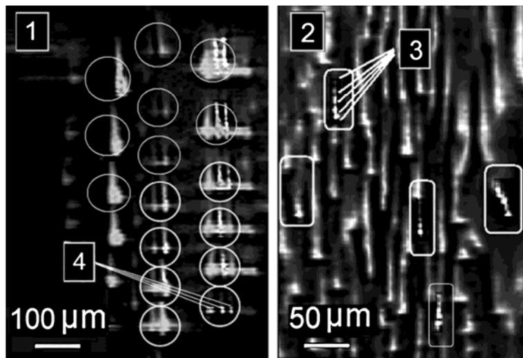
Fig. 4 – Fragments of images of dust structures (axial section) in cryogenic plasma: ordered clusters (1), the homogeneous structures formed out of threadlike clusters (2), single particles in threadlike cluster (3), flat cluster (4).
