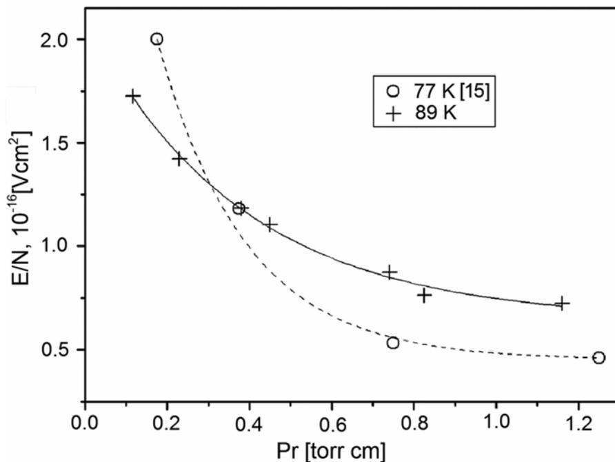
Fig. 3 – The reduced electric field  $E/N$  in a positive column depending on reduced pressure  $P_r$ , at cryogenic temperature at a discharge current  $I = 3$  mA.
