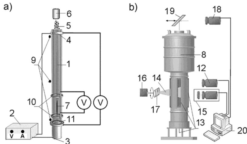
Fig. 1 – Reconstruction of experimental setup: discharge tube and scheme of electrical measurements (a) optical cryostat and scheme of the optical measurements (b).
