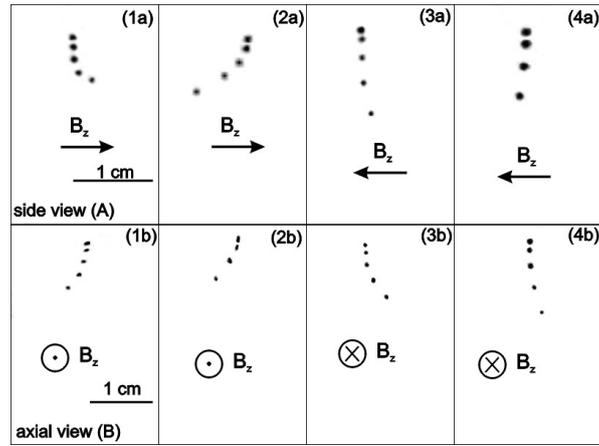
Fig. 2 – Each color inverted image shows a single dust particle captured in 4 or 5 frames: (a) are side images and (b) are axial images.
