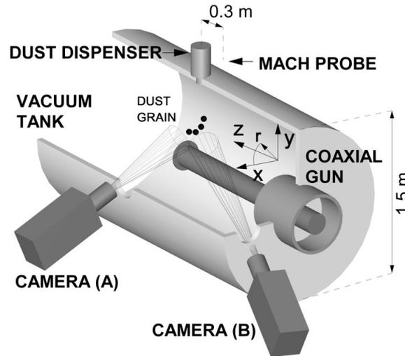
Fig. 1 – Coaxial plasma gun, dust dropper and high speed cameras, not to scale.
