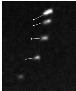
Fig. 4 – Dust particle captured by the CCD at successive times: the inclination of the dust trace with the horizontal is modified in time.
