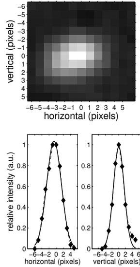
Fig. 3 – Gaussian fit for light emission of a dust particle captured by the CCD and visible pixels of the camera.
