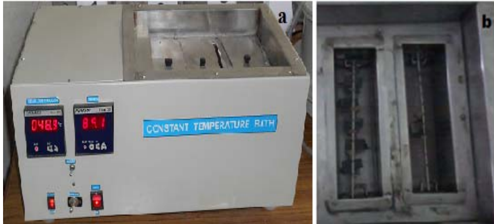
Fig. 1 – a) Constant temperature water bath; b) sample etching arrangement in the water bath.
