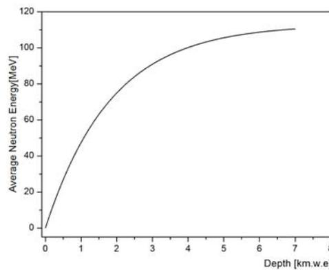
Fig. 3 – Average neutron energy as a function of depth.
