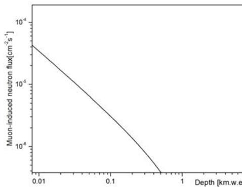
Fig. 4 – Muon-induced neutron flux as a function of depth.
