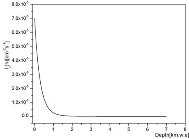
Fig. 2 – Differential muon intensity as a function of depth.
