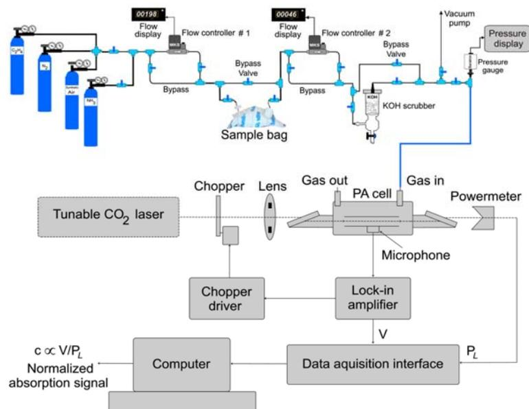
Fig. 1 – CO<sub>2</sub> laser photoacoustic spectroscopy system.
