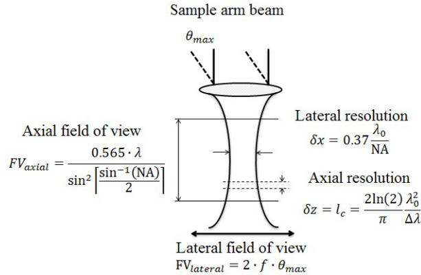
Fig. 2 – Schematic view over the sample arm of a general OCT system. Formulas depicted are assumed for axial field of view  $FV_{axial}$  and lateral resolution  $\delta_x$  (quantities dominated by confocal geometrical optics), axial resolution  $\delta_z$  (limited by the low-coherence interferometer) and lateral field of view  $FV_{lateral}$  (for a simple scanning system).
