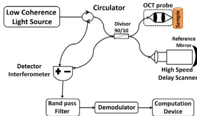
Fig. 1 – Fiber optic Michelson interferometer based OCT system.
