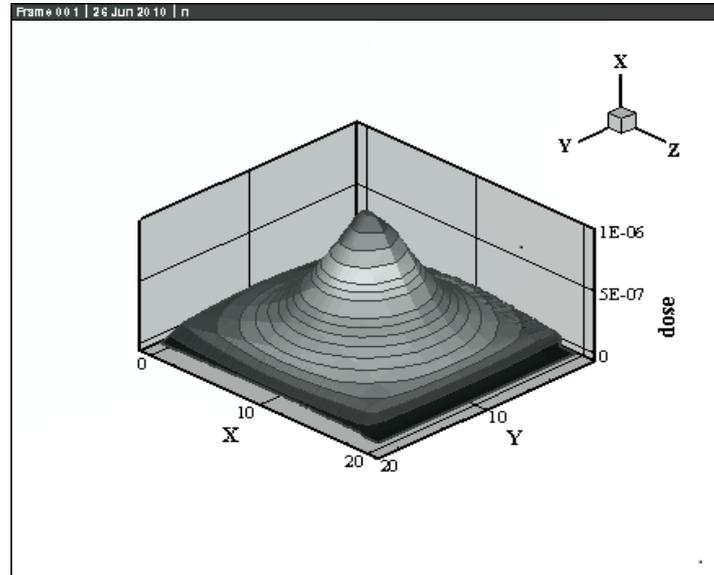
Fig. 7 – 3D dose distribution in PMMA phantom.
