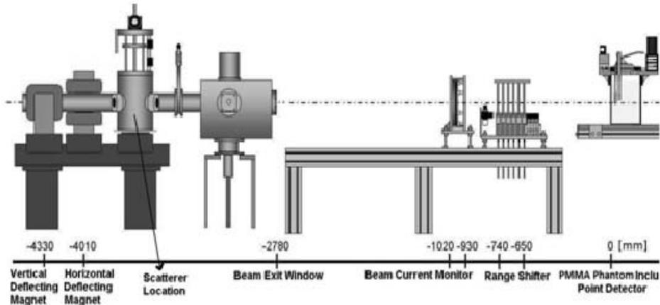
Fig. 1 – Schematic layout of proton beam path in Proton therapy facility, CYRIC [8].
