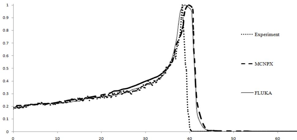
Fig. 2 – Percentage depth dose in PMMA phantom; Monte Carlo Simulation vs. experimental result.
