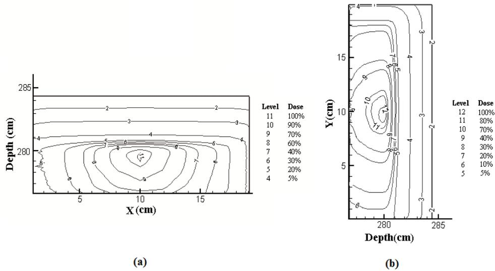
Fig. 5 – Isodose curves in X-Z plane (a) and in Y-Z plane (b), plotted by MCNPX (tecplot).
