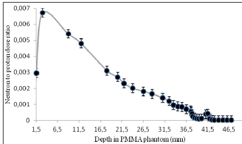
Fig. 8 – Ratio of neutron dose to proton dose in PMMA phantom.
