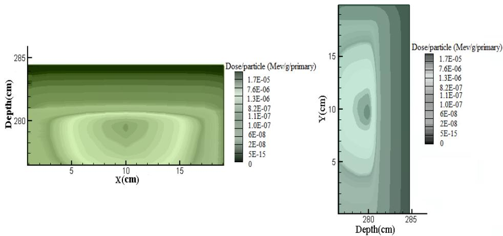
Fig. 6 – 2D dose distribution in PMMA phantom X-Z plane (a) and Y-Z plane (b), plotted by MCNPX (tecplot)
