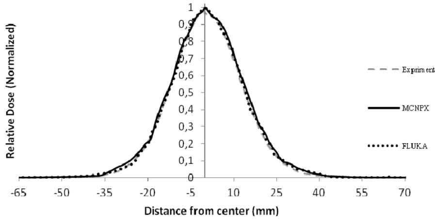
Fig. 3 – Lateral dose profile for pencil beam in longitudinal direction. Comparison between experimental data and Monte Carlo simulation. The solid line corresponds to the measured data; the round dot and dash present dose profile as calculated with FLUKA and MCNPX results respectively.
