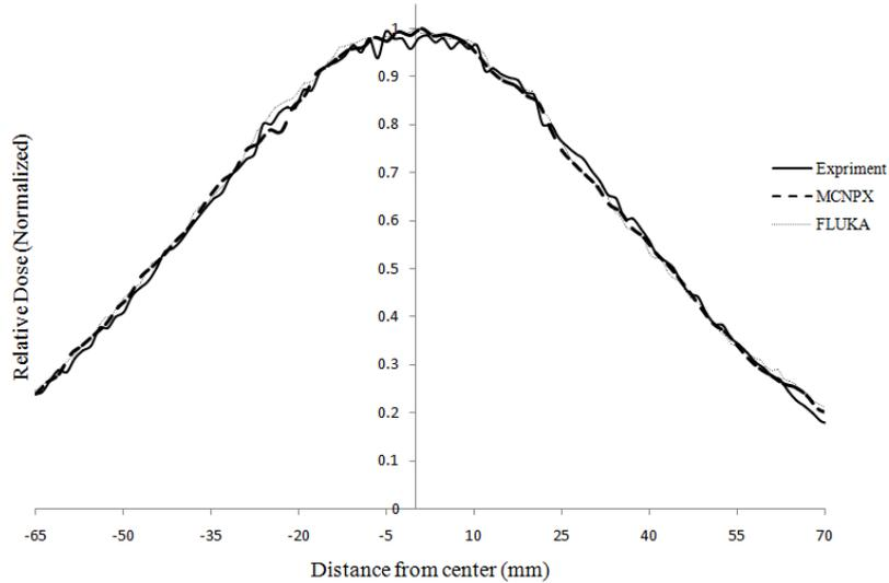
Fig. 4 – Lateral dose profile of flat beam in longitudinal direction. The results have been compared between Monte Carlo method and data from experiment. Again, solid line shows the measured data; the round dot and dash correspond to the dose profile as calculated with FLUKA and MCNPX results respectively.
