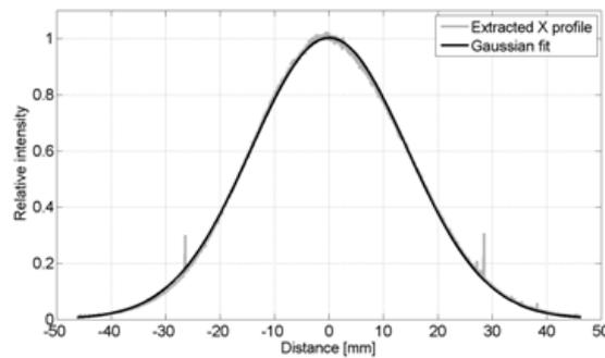
Fig. 9 – Profile X extracted from the acquired image of the non-scattered beam (gray line) and its Gaussian fit (black line). The distance from the ion guide to the scintillator screens was 215.1 cm.
