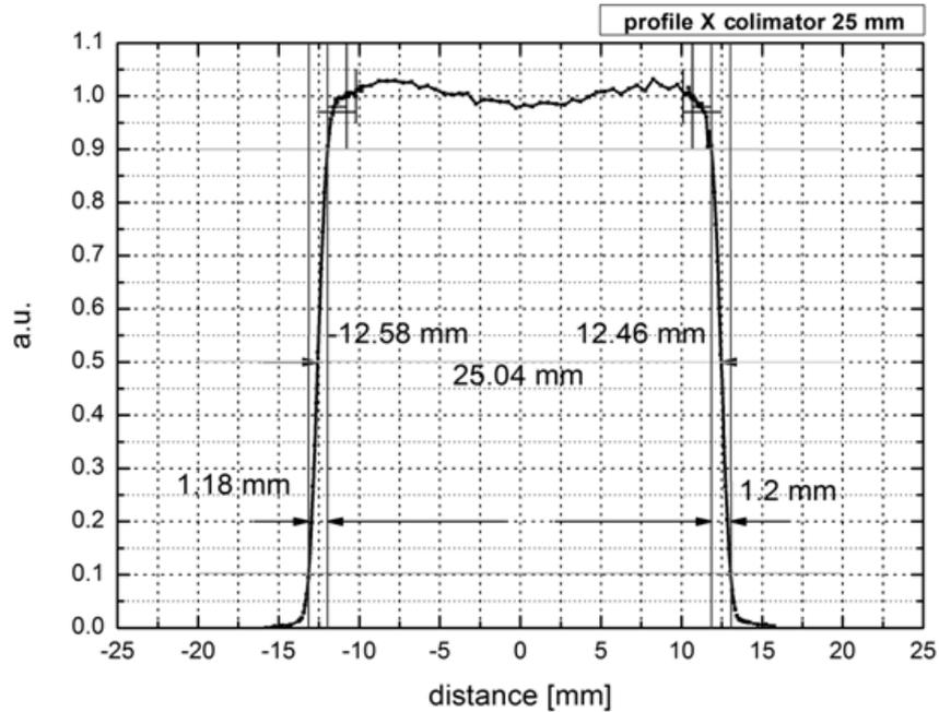
Fig. 3 – Result of the Profile Scanner measurements.
