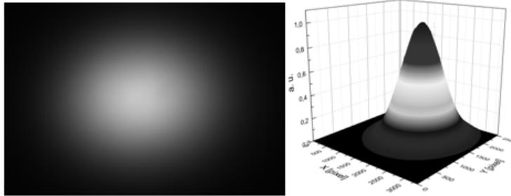
Fig. 8 – Image presented raw data recorded with the ProBImS (left) and a three dimensional reconstruction of the proton radiation intensity (right).
