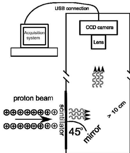
Fig. 4 – Layout of the beam scanning system.
