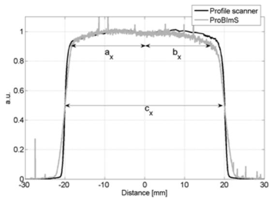
Fig. 7 – Profiles acquired *via* Profile Scanner with silicon diode (black) and ProBImS (gray).
