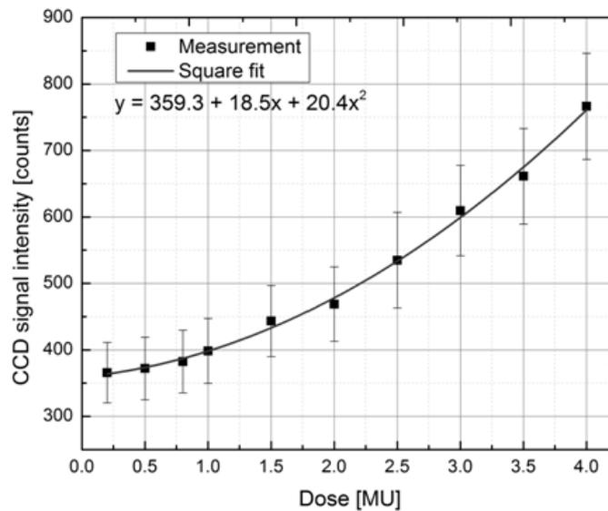
Fig. 5 – Background level as a function of absorbed dose.
