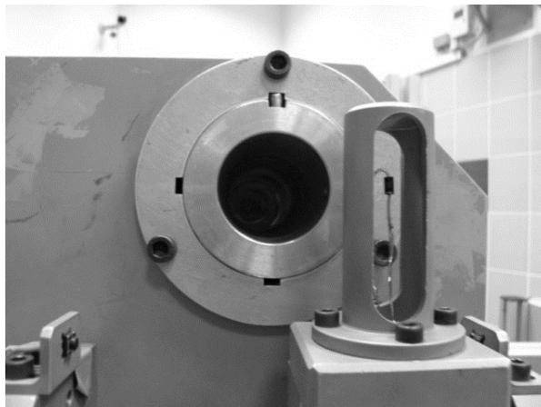
Fig. 2 – Profile Scanner with silicon diode.
