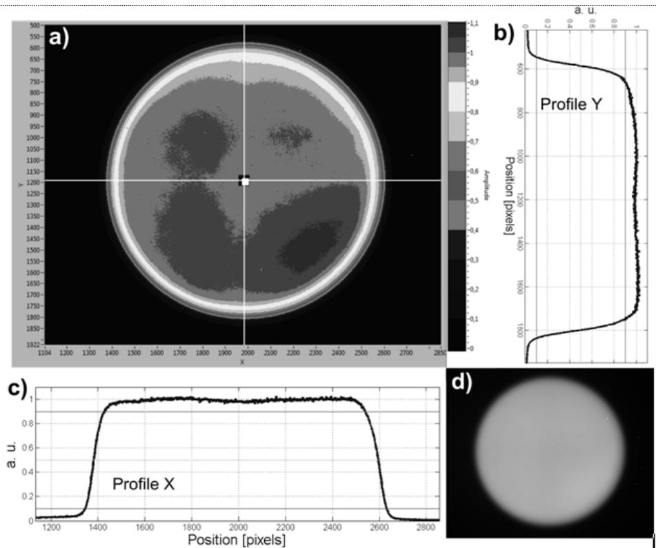
Fig. 6 – a) 2-dimensional beam spatial distribution recorded with the new system, using the  $\text{Gd}_2\text{O}_2\text{S:Tb}$  scintillator; b) vertical cross-section; c) horizontal cross-section; d) raw grayscale image of the beam.
