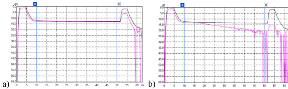
Fig. 3 – Measured spectra with wavelengths of 850 nm (black) and 1300 nm (red). In a) the optical fiber attenuation is measured before high energy photon beam irradiation, and b) after 400 Gy high energy photon beam exposure.
