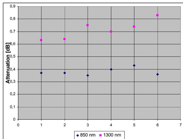
Fig. 1 – Optical Fiber attenuation before photon beam exposure.
