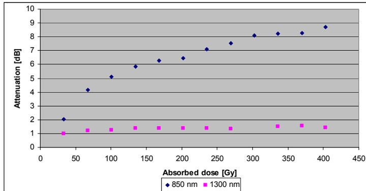
Fig. 2 – Optical Fiber attenuation while the fiber was exposed to high energy photon beam.
