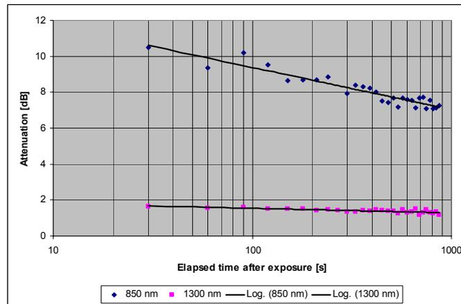
Fig. 5 – Optical fiber attenuation after an elapsed time [s].
