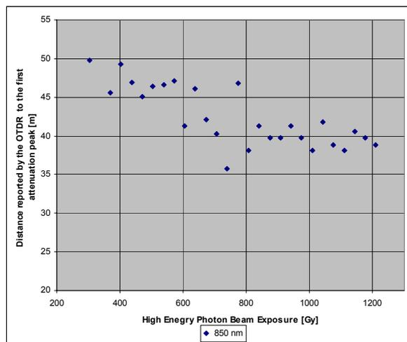
Fig. 4 – Distance reported by the OTDR to the first attenuation peak.
