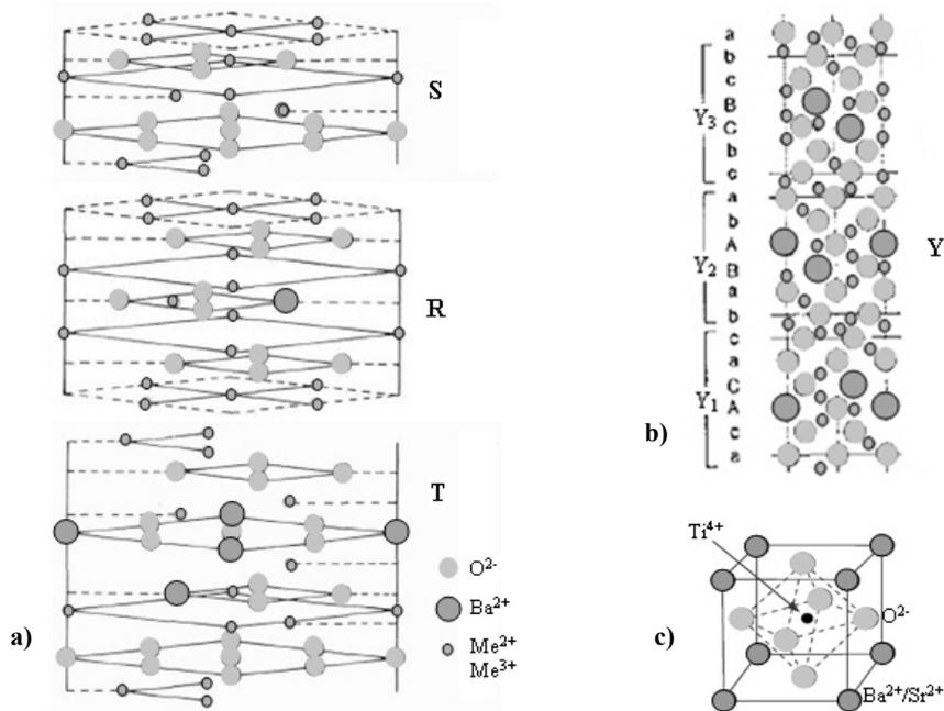
Fig. 2 – a) The S, R, T structural blocks included in the hexaferrites. Blocks can be rotated in a succession specific to each configuration ( $M, Y, Z$ ); b) the crystallographic build up of the Y type hexaferrites; a, b, c – close-packed oxygen layers; A, B, C – mixed Ba-O layers (after van Landuyt *et al.*, 1974); c) the perovskite structure of the ferroelectric phase,  $\text{Ba}_x\text{Sr}_{1-x}\text{TiO}_3$ .
