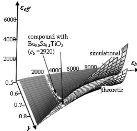
Fig. 3 – Effective permittivity evolution *versus* ferroelectric phase permittivity and concentration, for the nanocomposite with *M* type hexaferrite ( $\epsilon_{a,M} = 8.18 = \text{ct.}$  for  $\text{Ba}_{0.8}\text{Sr}_{0.2}\text{Fe}_{12}\text{O}_{19}$ ).
