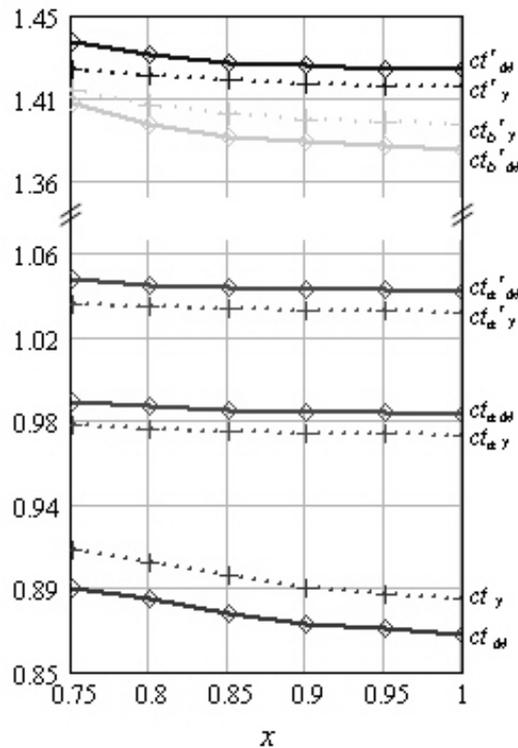
Fig. 7 – Evolution of the derived mixture law coefficients for effective permittivity of the nanocomposite versus the substitution degree in the ferroelectric phase. Coefficients are given for the combinations with  $M$ , respectively  $Y$  hexaferrite.
