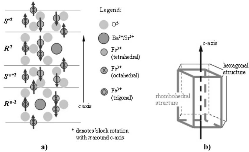
Fig. 1 – a) The RSR\*S\* block structure of the Ba-M hexaferrite, with the spin configuration. The easy magnetization direction is along the crystallographic  $c$ -axis; b) hexagonal / rhombohedral structure with the  $c$  magnetization axis.
