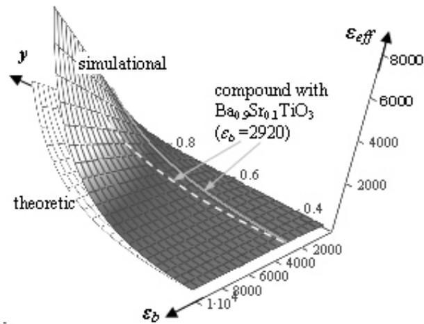
Fig. 5 – Effective permittivity evolution *versus* ferroelectric phase permittivity and concentration, for the nanocomposite with *Y* type hexaferrite ( $\epsilon_{a,Y} = 16.2 = ct.$  for  $Ba_2Zn_2Fe_{12}O_{22}$ ).
