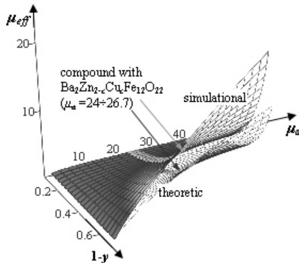
Fig. 6 – Effective permeability evolution *versus* ferrite phase permeability and concentration, for the nanocomposite with *Y* type hexaferrite; the perovskite ( $Ba_{0.9}Sr_{0.1}TiO_3$ ) has no magnetic properties ( $\mu_b = 1 = ct.$ ).
