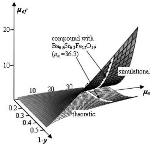
Fig. 4 – Effective permeability evolution *versus* ferrite phase permeability and concentration, for the nanocomposite with *M* type hexaferrite; the perovskite ( $\text{Ba}_{0.9}\text{Sr}_{0.1}\text{TiO}_3$ ) has no magnetic properties ( $\mu_b = 1 = \text{ct.}$ ).
