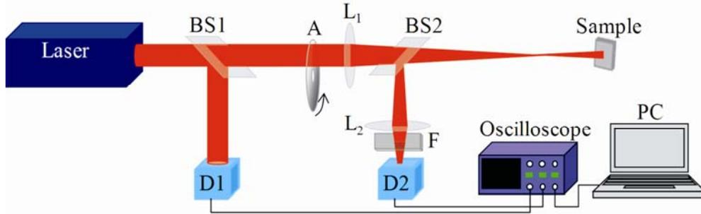
Fig. 1 – RI-scan experimental setup: laser, A – variable attenuator,  $L_1$ ,  $L_2$ - lenses, BS1, BS2 – beam-splitters, D1, D2 – detectors, F – neutral filter.
