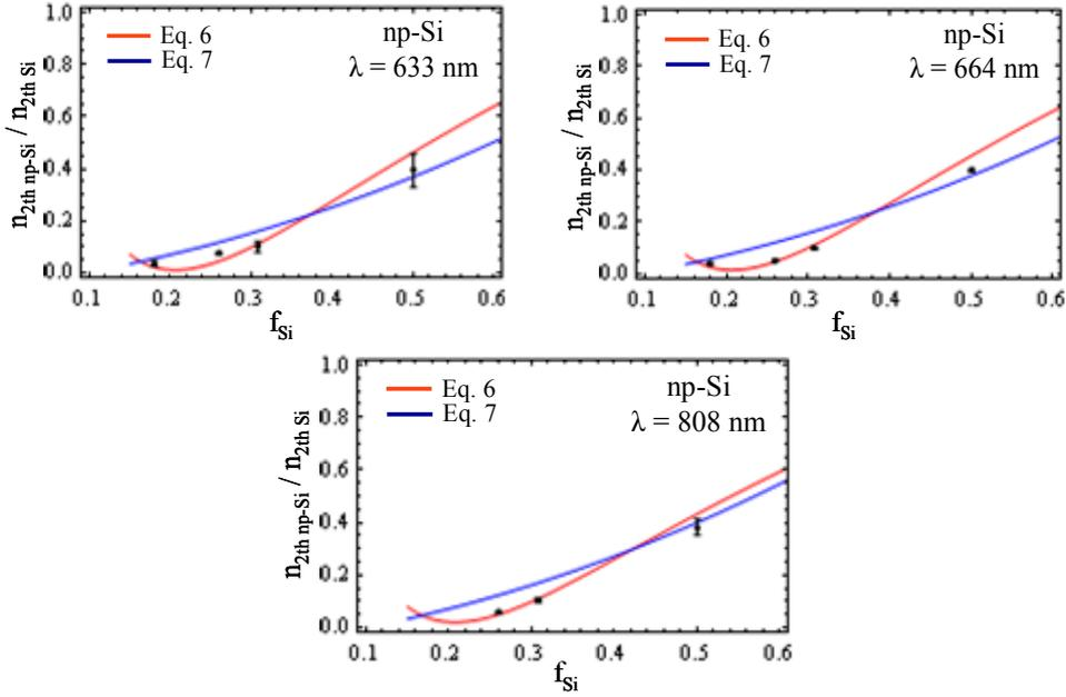
Fig. 3 – Dependences of  $n_{2, np-Si}/n_{2, Si}$  on the Si volume fill fraction (at fixed wavelengths, in c.w. regime)
