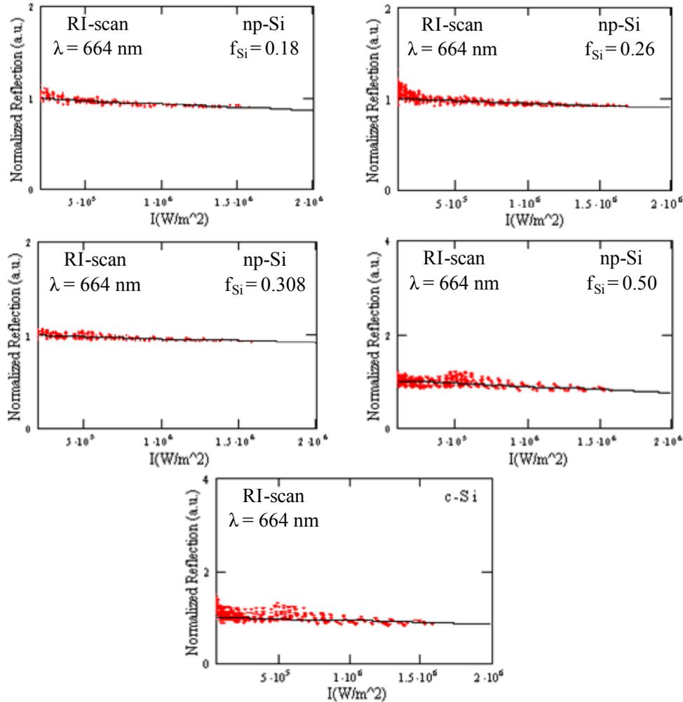
Fig. 2 – RI-Scan experimental data and for nano-porous silicon layers with different  $f_{Si}$  and for bulk Si (c-Si), at 664 nm excitation wavelength.
