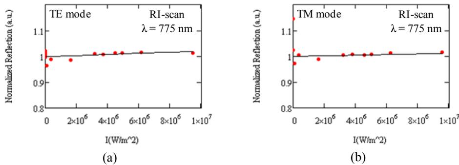
Fig. 4 – RI-Scan experimental data for 1D periodic SOI nanostructures, at  $\lambda = 775$  nm in fs pulsed regime, for TE mode (a) and TM mode (b).
