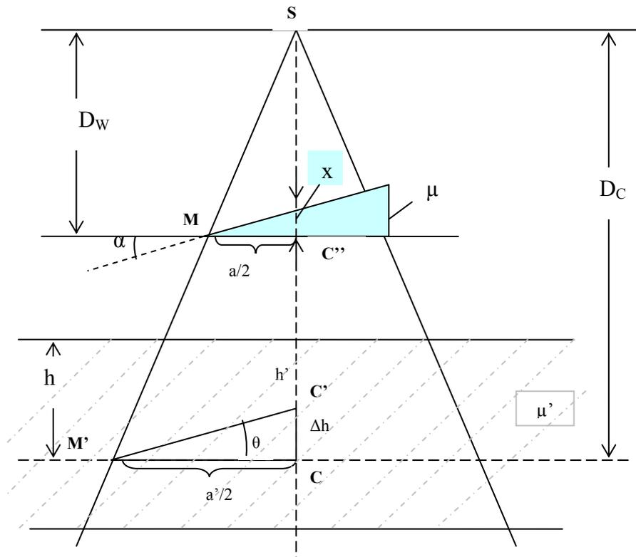
Fig. 1 – Irradiation's geometry; S – radioactive source position;  $\alpha$  – wedge angle;  $\mu$  – absorption coefficient of wedge material,  $\mu = 0.640 \text{ cm}^{-1}$ ;  $\mu'$  – attenuation coefficient of irradiated medium – water equivalent soft tissue,  $\mu' = 0.063 \text{ cm}^{-1}$ ;  $a'$  – irradiation field size;  $a$  – wedge length placed in beam;  $\theta$  – rotation angle of isodose plateau;  $D_w$  – wedge source distance;  $D_C$  – evaluation point-source distance.
