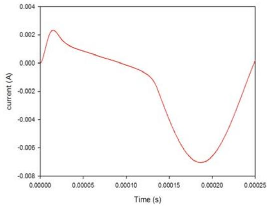
Fig. 4 – Evolution of the total discharge current in typical cycle.
