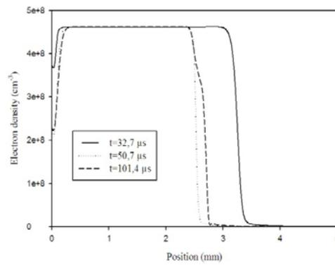
Fig. 10 – The spatial distribution of electron density in  $t = 32.7\mu\text{s}$ ,  $t = 50.7\mu\text{s}$  and  $t = 101.4\mu\text{s}$ .
