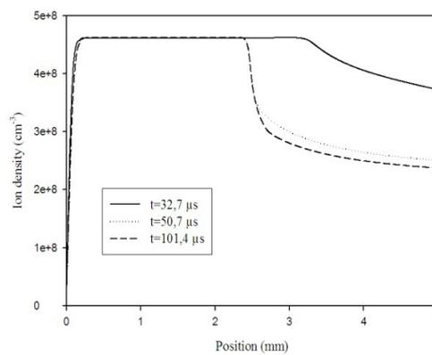
Fig. 11 – The spatial distribution of ion density in  $t = 32.7\mu\text{s}$ ,  $t = 50.7\mu\text{s}$  and  $t = 101.4\mu\text{s}$ .
