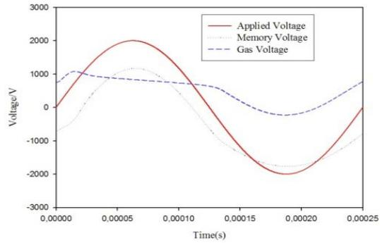
Fig. 3 – Evolution of the gas voltage in typical cycle.
