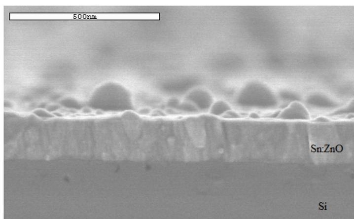
Fig. 4 – Cross-section SEM image of a Sn doped ZnO thin film grown by PED on Si substrate at 200°C.
