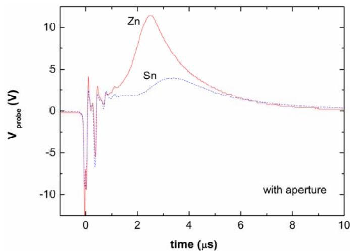
Fig. 2 – Ion probe signals for Zn ions (solid line) and Sn ions (dashed line).
