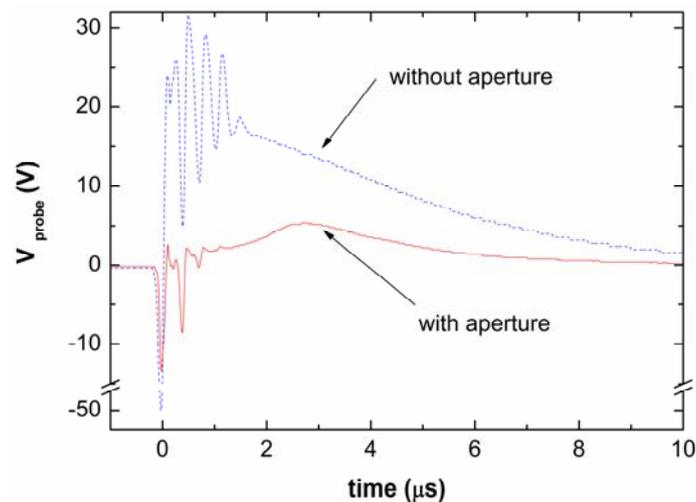
Fig. 1 – Ion probe signals recorded without aperture (dashed line) and with 1mm aperture (solid line).
