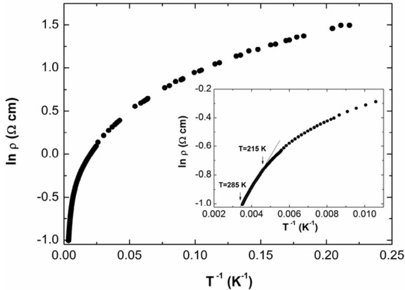
Fig. 5b – Arrhenius plot of the resistivity of a Sn doped ZnO thin film grown by PED on c-cut sapphire substrate at 200 °C. The inset shows the variation in the 285 to 215 K range on an expanded scale.
