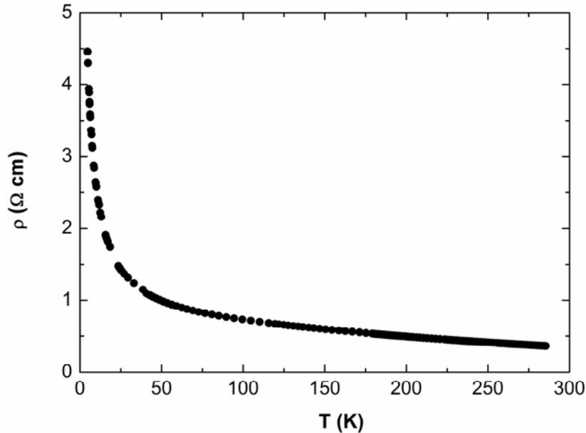
Fig. 5a – The resistivity as a function of temperature of Sn doped ZnO thin film grown by PED on c-cut sapphire substrate at 200°C.
