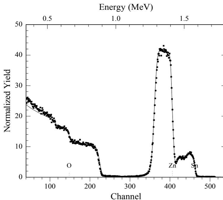
Fig. 3 – A typical RBS spectrum recorded for a Sn doped ZnO film grown by PED on c-cut sapphire substrate at 200°C.
