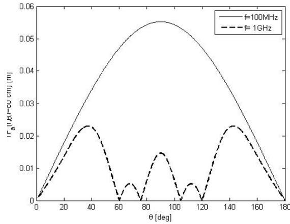
Fig. 4 – Transfer function a dipole antenna of 80 cm with  $\theta_a$  at two operating frequencies: continuous line-100MHz, dashed line-1GHz.
