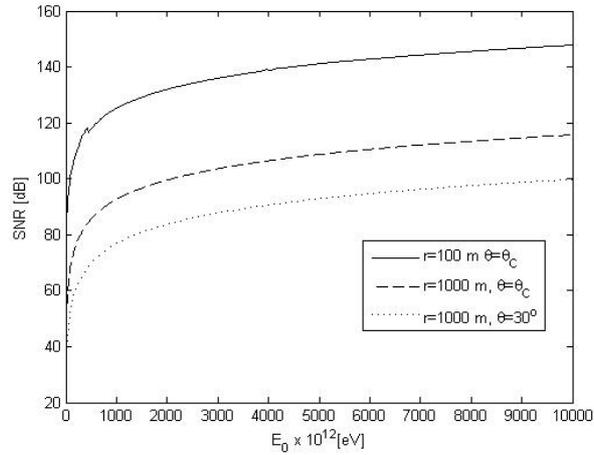
Fig. 7 – SNR as function of the energy of the primary particle. We have presented with a dashed line the SNR at  $\theta_c$  at  $1\,000\text{ m}$ ; with a continuous line—at  $100\text{ m}$ . The dotted line represents SNR at  $1\,000\text{ m}$  with  $\theta = 30\text{ deg.}$  We have assumed  $\theta_a = 30\text{ deg.}$
