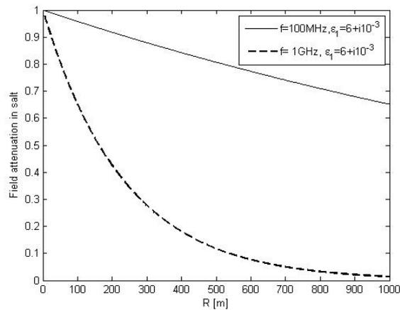
Fig. 3 – The field attenuation as function of the propagation distance. The dashed line represents the situation when  $f=100\text{MHz}$  and the continuous one, at 1 GHz.
