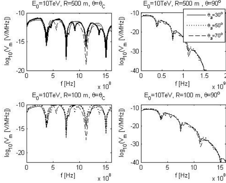
Fig. 6 – Voltage delivered to the load. The upper panels present the situation when the distance between antenna and receiver is 500 m and the lower panel –  $R = 100$  m. The plots on the left side show observations at the Cherenkov angle and the lots on the side show observations at the 90 deg.
