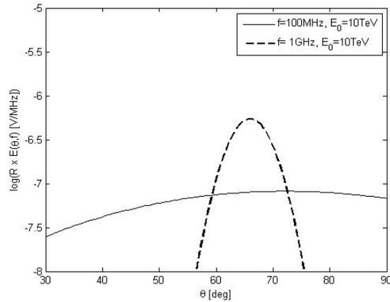
Fig. 2 – The  $E$ -field generated by a 10TeV particle as function of the observation angle. The dashed line describes a 1 GHz operating frequency; the continuous line – 100 MHz.
