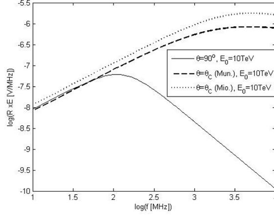
Fig. 1 – The  $E$ -field generated by a 10TeV particle at the Cherenkov angle as function of the operating frequency. The dashed line describes the parameterization in [10]; the dotted line – the parameterization in [23]. Both cases are at Cherenkov angle. The continuous line presents the parameterization in [10] at an observation angle of 90 deg.
