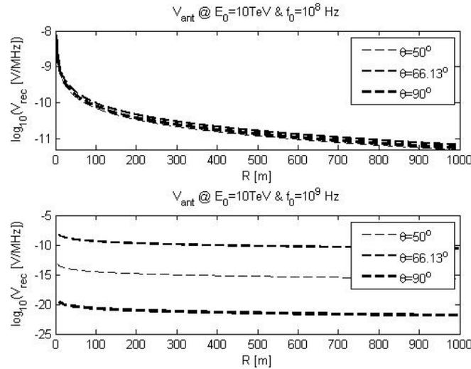
Fig. 5 – Voltage on the antenna as function of the distance between the shower and antenna, for an  $E$ -field generated by a 10TeV particle. The upper panel presents the situation of an operating frequency of 100MHz and the lower panel, an operating frequency of 1GHz. Both cases present different observation angles: 50 deg. (thin line), 66.13 deg. (thicker line) and 90deg. (thickest line).
