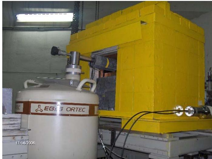
Fig. 4 – Back view of the low-background spectrometer showing the Ge(Li) measuring the background inside of lead castle.
