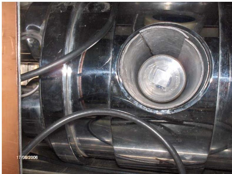
Fig. 3 – Back view of the low-background spectrometer showing the  $4\pi$  NaI(Tl) summing detector and the plexiglass plug for target supporting.
