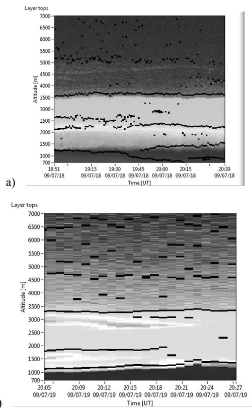
Fig. 9 – Range Corrected Signal time series and layer top retrieved from lidar on:
