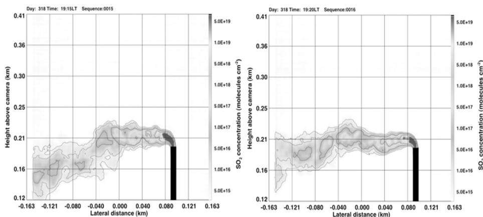
Fig. 1 – Some examples of plume stack  $\text{SO}_2$  measurements.
