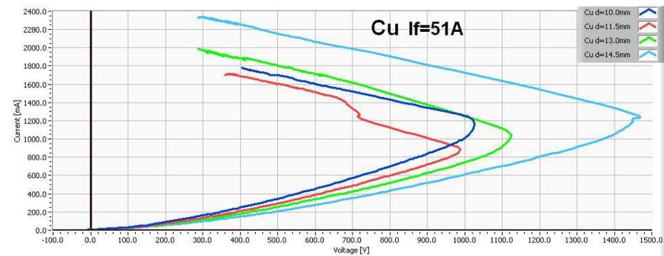
Fig. 2 – I-V characteristics for same heating filament current, different inter electrodes distance.
