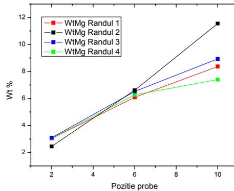
Fig. 8 – MgO concentration in respect with the substrate position.
