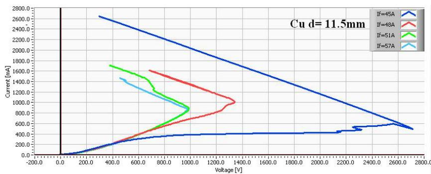
Fig. 3 – I-V characteristics for same inter electrodes distance, different heating filament current.
