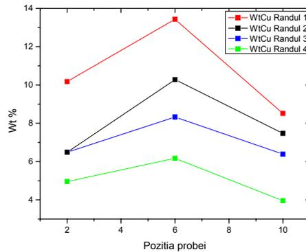
Fig.7 – Cooper concentration in respect with the substrate position.
