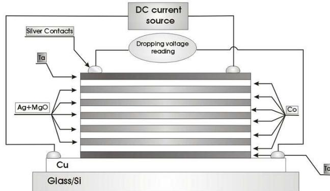
Fig. 9 – Electric four points measurement for the multilayer structure.
