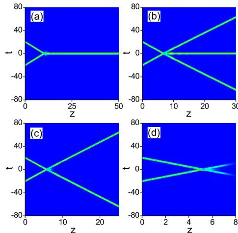
Fig. 1 – Contour plots display the evolution of the electric field in the plane  $(t, z)$  for on-site discrete Ginzburg-Landau light bullets localized at the edge of the waveguide array ( $d = 0$ ). Here  $\varepsilon = 3.5$ , and the kick parameter  $\chi = 2$  (a),  $\chi = 3$  (b),  $\chi = 3.6$  (c), and  $\chi = 4$  (d).
