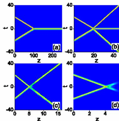
Fig. 7 – Trajectories of the  $(20, 20)$  center discrete Ginzburg-Landau light bullets, which correspond to soliton fusion (a), soliton birth (b), elastic collision (c), and soliton decay (d). Here  $\varepsilon = 3.7$ , and the kick parameter  $\chi = 0.2$  (a),  $\chi = 1$  (b), and  $\chi = 4$  (c), and  $\chi = 5$  (d).
