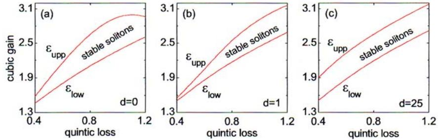
Fig. 2 – Domains of existence and stability in the plane  $(\mu, \epsilon)$  for on-site dissipative discrete surface light bullets located at distances of: a)  $d = 0$ ; b)  $d = 1$ ; c)  $d = 25$  from the edge of the waveguide array. Here the linear loss coefficient  $\delta = 1$ .
