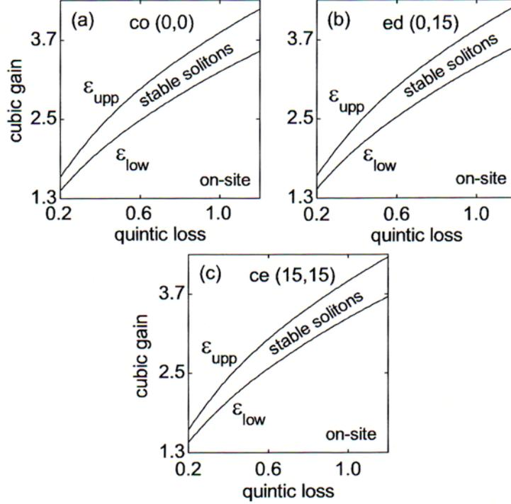
Fig. 7 – Domains of existence and stability in the plane  $(\mu, \varepsilon)$  for on-site dissipative discrete light bullets located in the corner (co), at the edge (ed), and in the center (ce), respectively.
