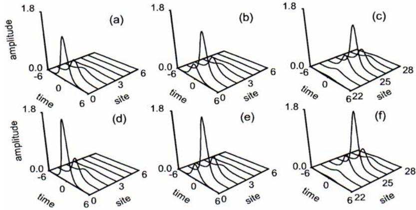
Fig. 1 – Examples of stable on-site discrete spatiotemporal surface solitons with both relatively low and relatively high peak amplitudes localized at distances of [(a) and (d)]  $d = 0$ , [(b) and (e)]  $d = 1$ , and [(c) and (f)]  $d = 25$  from the edge of the waveguide array. Here  $\delta = 1$ ,  $\mu = 1$ , and: a)  $\varepsilon = 2.365$ ; b)  $\varepsilon = 2.440$ ; c)  $\varepsilon = 2.462$ ; d)  $\varepsilon = 2.953$ ; e)  $\varepsilon = 2.914$ ; f)  $\varepsilon = 2.930$ .
