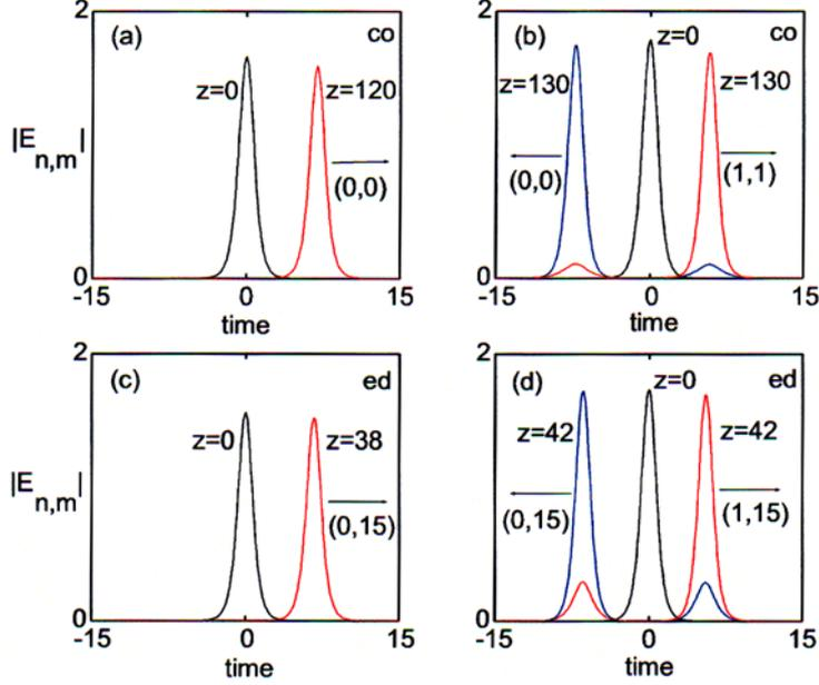
Fig. 8 – Reshaping of the relatively low-amplitude unstable inter-site (a) (0, 0) corner and (c) (0, 15) edge solitons into moving low-energy on-site corner and edge solitons, respectively, centered at the same lattice sites, and splitting of the relatively high amplitude unstable inter-site (b) corner and (d) edge solitons into two moving in opposite directions on-site solitons localized at different lattice sites. Here  $\mu = 1$ ,  $\varepsilon = 3.3$  (a,c), and  $\varepsilon = 3.5$  (b,d).
