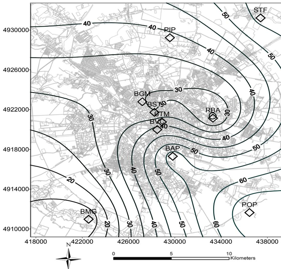
Fig. 1 – Map of the interpolated values of PGA\_EW [ $\text{cm/s}^2$ ] in Bucharest for the earthquake of 27.10.2004. Coordinates are in UTM. Diamond symbols represent the seismic station locations.
