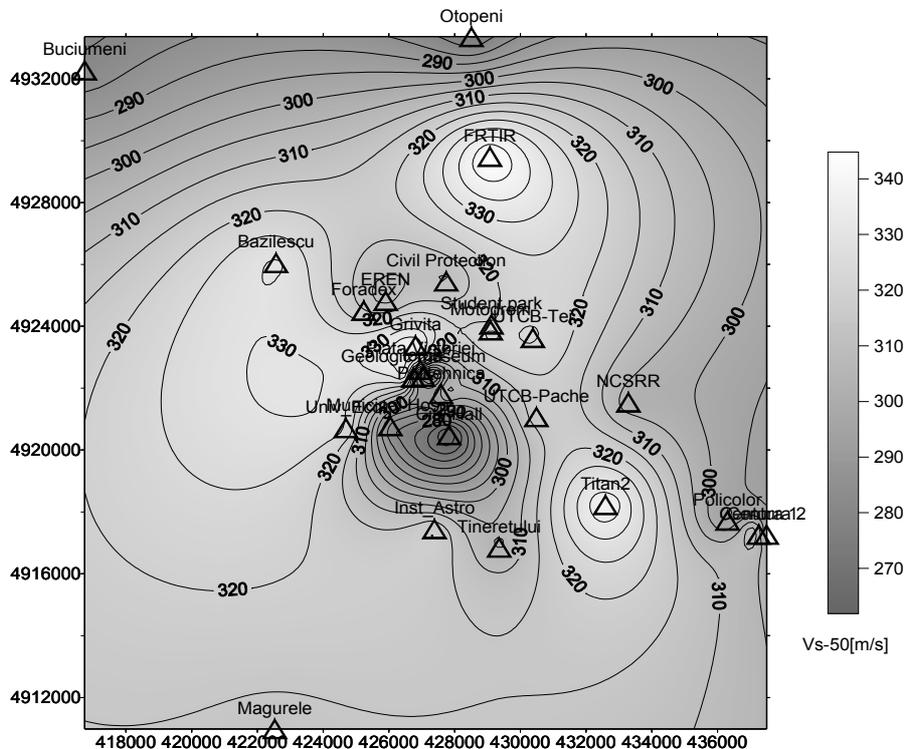
Fig. 5 – Map of the mean weighted seismic velocity ( $V_{s-50}$ ) in Bucharest City from downhole seismic measurements. Coordinates are given in UTM system (meters).
