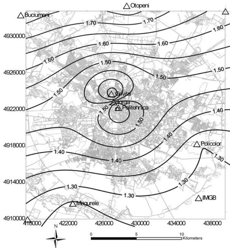
Fig. 3 – Map of the characteristic site period for the Bucharest City. Coordinates are given in UTM system [meters]. Borehole sites are represented by triangles.
