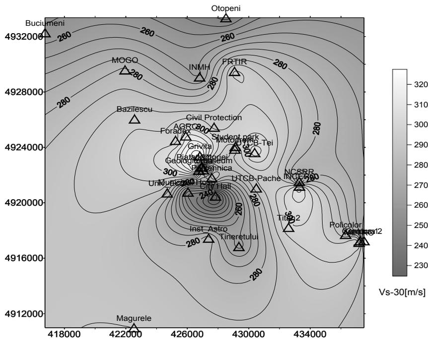
Fig. 4 – Map of the mean weighted seismic velocity ( $V_{S-30}$ ) in Bucharest City from downhole seismic measurements. Coordinates are given in UTM system (meters).
