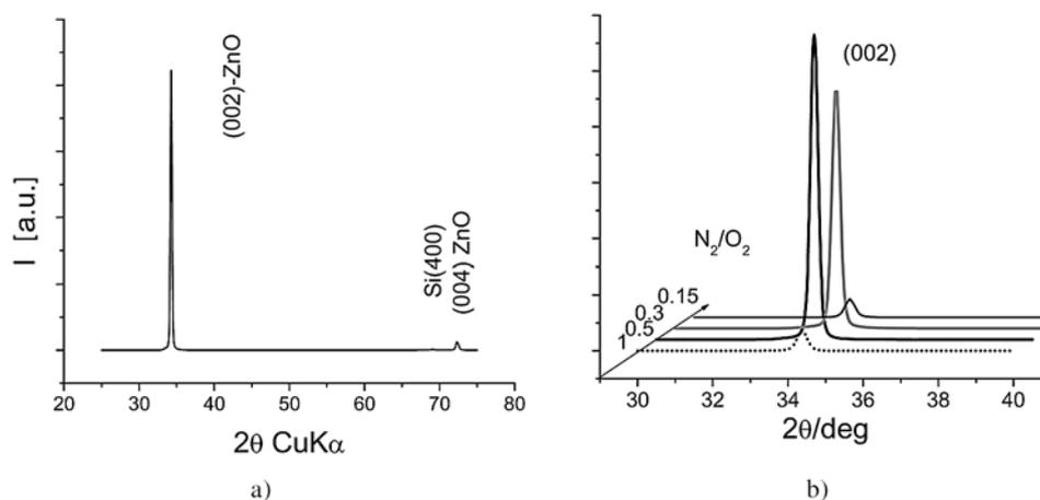
Fig. 9 – Representative XRD pattern of a nitrogen-doped ZnO film (N<sub>2</sub>/O<sub>2</sub> = 0.3 in the gas mixture) (a) and (002) peak at various concentrations of nitrogen in the gas mixture (b).
