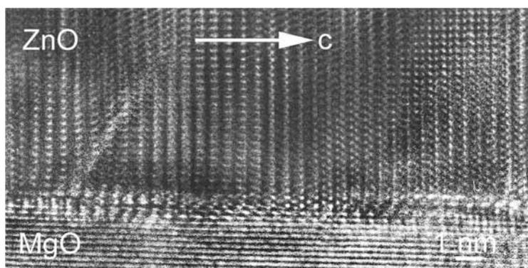
Fig. 7 – High resolution TEM in cross section of the interface between the  $a$  axis oriented ZnO layer grown on MgO single crystal.
