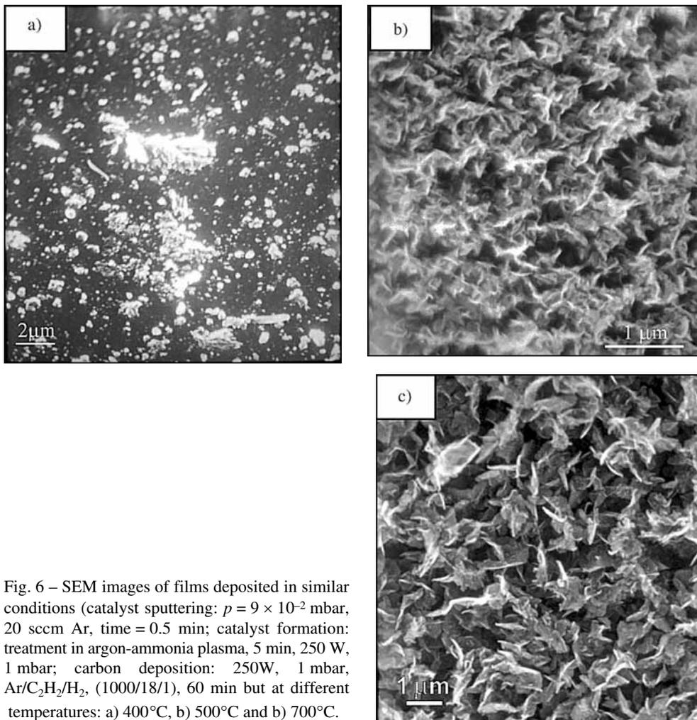
Fig. 6 – SEM images of films deposited in similar conditions (catalyst sputtering:  $p = 9 \times 10^{-2}$  mbar, 20 sccm Ar, time = 0.5 min; catalyst formation: treatment in argon-ammonia plasma, 5 min, 250 W, 1 mbar; carbon deposition: 250W, 1 mbar, Ar/C<sub>2</sub>H<sub>2</sub>/H<sub>2</sub>, (1000/18/1), 60 min but at different temperatures: a) 400°C, b) 500°C and c) 700°C.
