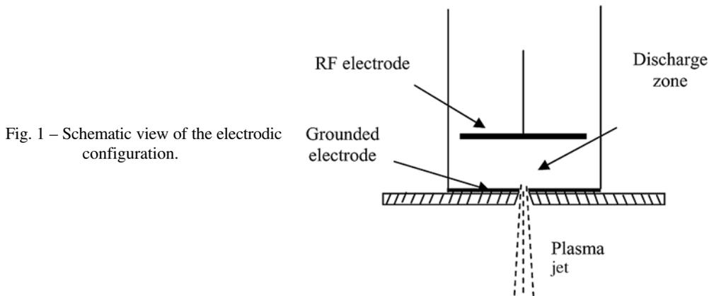
Fig. 1 – Schematic view of the electrode configuration.
