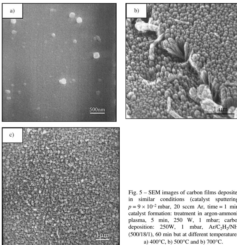
Fig. 5 – SEM images of carbon films deposited in similar conditions (catalyst sputtering:  $p = 9 \times 10^{-2}$  mbar, 20 sccm Ar, time = 1 min; catalyst formation: treatment in argon-ammonia plasma, 5 min, 250 W, 1 mbar; carbon deposition: 250W, 1 mbar, Ar/C<sub>2</sub>H<sub>2</sub>/NH<sub>3</sub> (500/18/1), 60 min but at different temperatures: a) 400°C, b) 500°C and b) 700°C.
