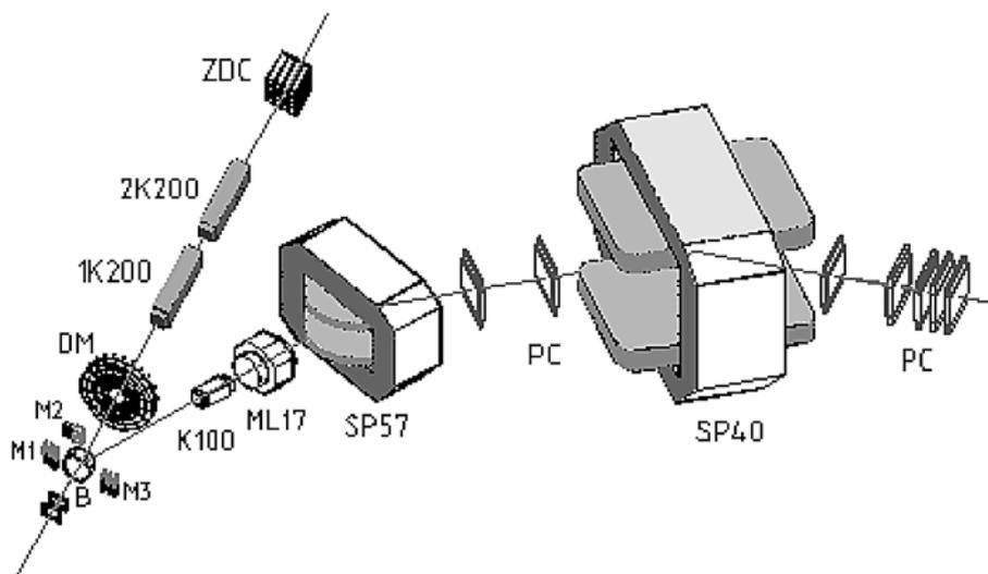
Fig. 1 – MARUSYA experimental set up – large view.
