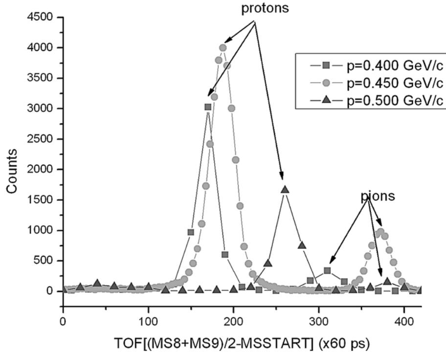
Fig. 4 – The TOF distributions of pions and protons for three modes of operation of the spectrometer.
