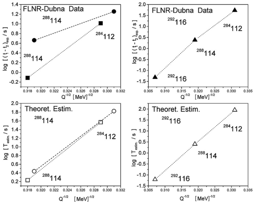
Fig. 2 – Summary of the  $\alpha$ -decay data obtained by Oganessian *et al.* [40–42] for  $^{287-289}_{114}$  isotopes and estimated  $\alpha$ -half-lives.
